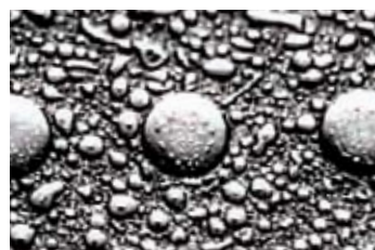
MT Connector Cleaned with IPA
