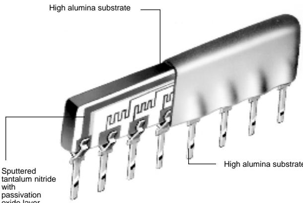
The solution to increasing precision resistor component density, economically, is IRC's commercial SMXX Series SIP Ultra Precision Resistor Network. This small footprint, conformally coated SIP features three (3) standard sizes (6, 8, 10 pin versions) and three (3) different circuits schematics and is only 0.250" high.
