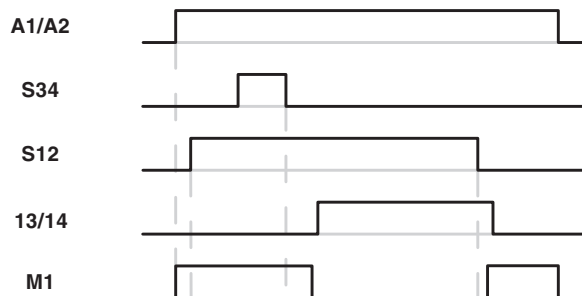
Figure 6 Time diagram PSR-MS25
