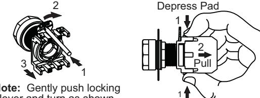
**Transformer Units Assembly**
