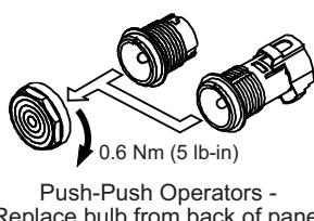
Push-Push Operators - Replace bulb from back of panel
