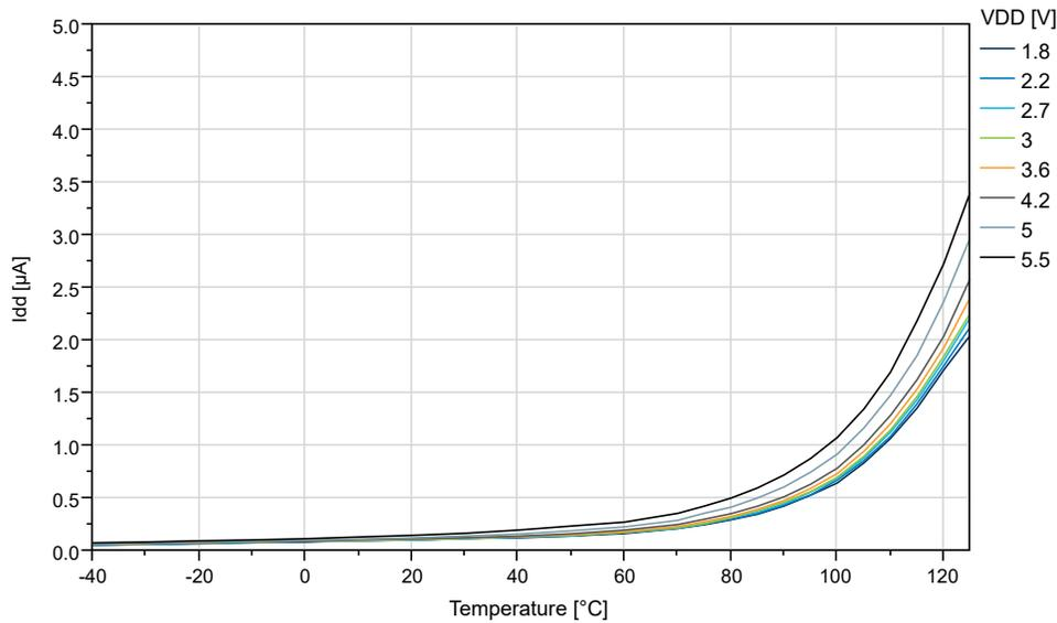
**Figure 32-11. ATtiny204/ATtiny404: Power-Down Mode Supply Current vs.  $V_{DD}$  (All Functions Disabled)**
