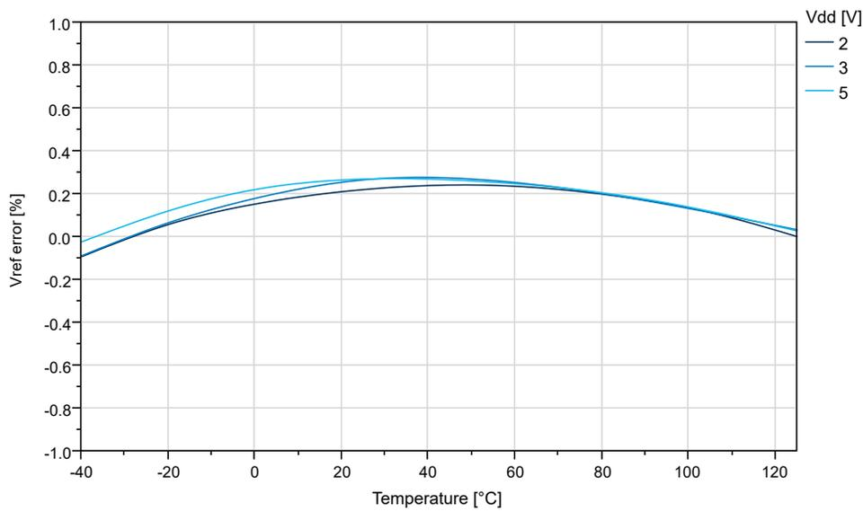
**Figure 32-33. Internal 2.5V Reference vs. Temperature**
