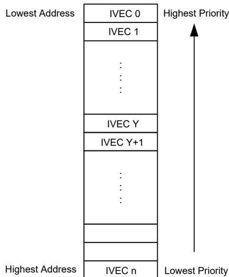
The default priority can be changed by writing to the CPUINT.LVL0PRI register. The value written to the register will identify the vector number with the lowest priority. The next interrupt vector in IVEC will have the highest priority, see the following figure. In this figure, the value Y has been written to
