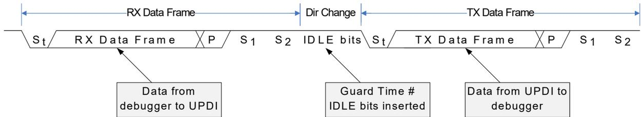
The UPDI Guard Time is the minimum IDLE time that the connected debugger will experience when waiting for data from the UPDI. Because of the asynchronous interface to the system, as presented in [Clocks](#), the ratio between the UPDI clock and the system clock will affect the synchronization time, and how long it takes before the UPDI can transmit data. In the cases where the synchronization delay is shorter than the current Guard Time setting, the Guard Time will be given by GTVAL directly.
