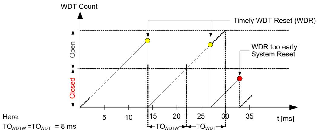
The Window mode is enabled by writing a non-zero value to the WINDOW bit field in the Control A register (WDT.CTRLA), and disabled by writing WINDOW=0x0.
