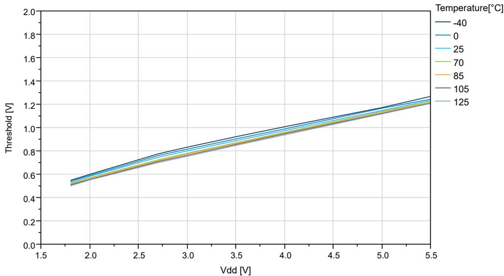
**Figure 32-17. I/O Pin Input Threshold Voltage vs.  $V_{DD}$  ( $T=25^{\circ}\text{C}$ )**
