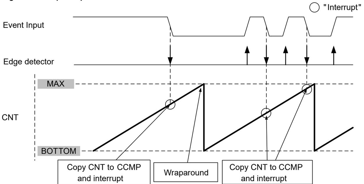
It is recommended to write '0' to the TCBn.CNT register when entering this mode from any other mode.
