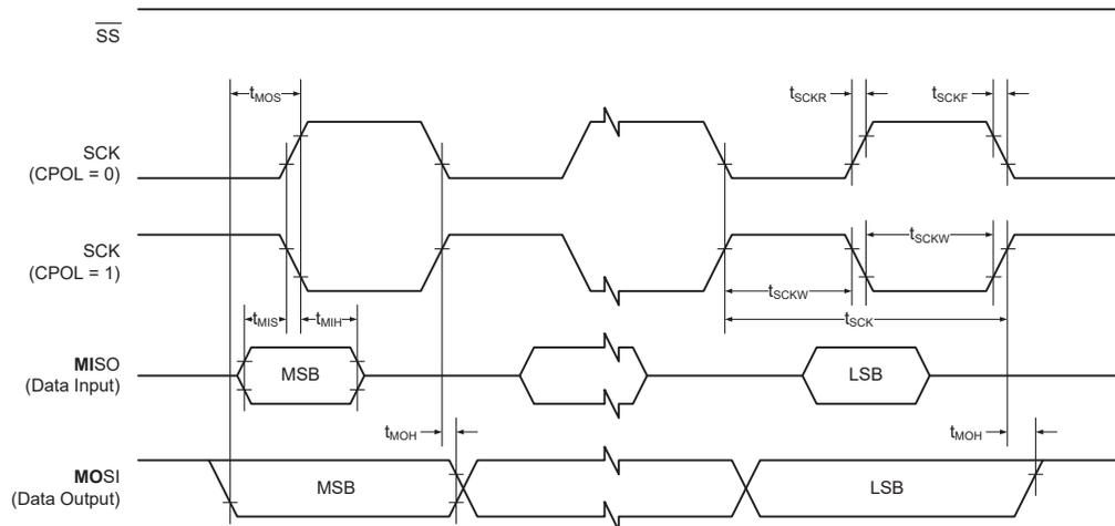
**Figure 31-5. SPI - Timing Requirements in Slave Mode**
