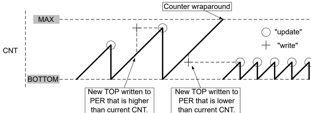
A counter wraparound can occur in any mode of operation when up-counting without buffering. This is due to the fact that the TCA<sub>n</sub>.CNT and TCA<sub>n</sub>.PER registers are continuously compared: if a new TOP value is written to TCA<sub>n</sub>.PER that is lower than current TCA<sub>n</sub>.CNT, the counter will wrap first, before a compare match happens.
