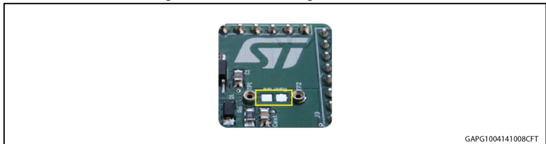
Figure 5: Pads for soldering SMD resistor
