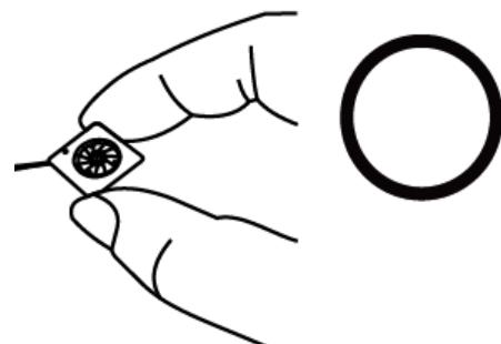
Don't pull fan with lead wires.
