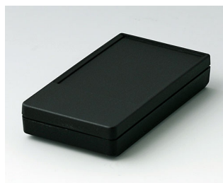
A9070219 DATEC-POCKET-BOX S PMMA (IR) (UL 94 HB) black RAL 9005 3.35"x1.81"x0.63" IP 54
