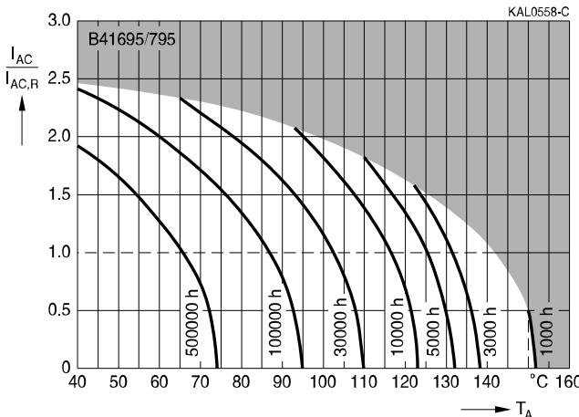
**Useful life<sup>1)</sup>**depending on case temperature  $T_C$  under ripple current operating conditions at  $V_{op}$
