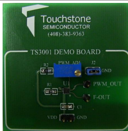
Figure 2. TS3001 Evaluation Board
