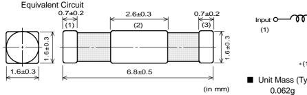
Output (3) **GND** (2) \*(1),(3):No Polarity
