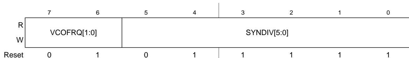
Figure 7-4. S12CPMU Synthesizer Register (CPMUSYNR)
