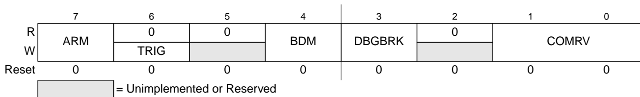
Figure 6-3. Debug Control Register (DBG1)
