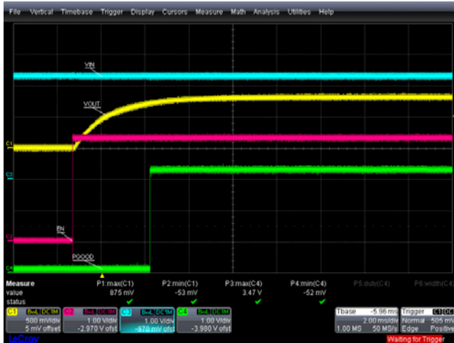
FIGURE 21. POWER-ON AND POWER-OFF, EN = 0 TO 1, +25°C, VIN = 6V, VOUT = 0.8V, IOUT = 0.5A, PGGOOD TURN-ON
