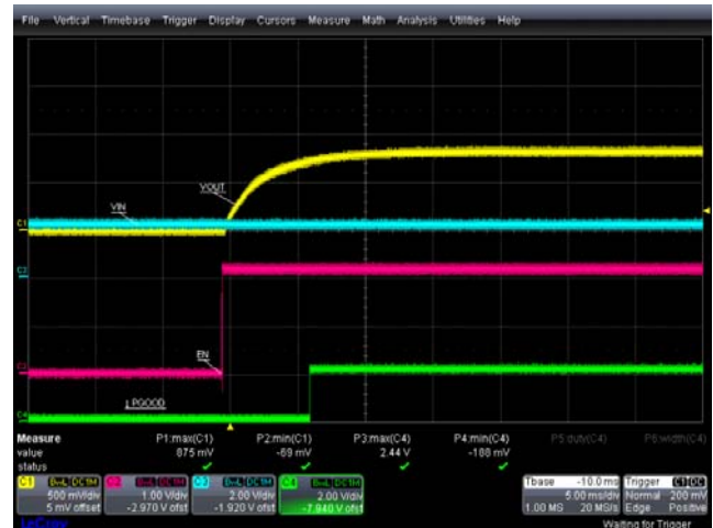
FIGURE 22. POWER-ON AND POWER-OFF, EN = 0 TO 1, +25°C, VIN = 2.2V, VOUT = 0.8V, IOUT = 0.5A, PGGOOD TURN-ON
