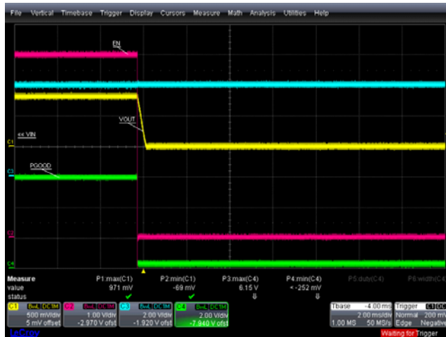
FIGURE 23. POWER-ON AND POWER-OFF, EN = 1 TO 0, +25°C, VIN = 6V, VOUT = 0.8V, IOUT = 0.5A, PGGOOD TURN-OFF
