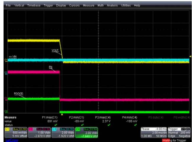
FIGURE 24. POWER-ON AND POWER-OFF, EN = 1 TO 0, +25°C, VIN = 2.2V, VOUT = 0.8V, IOUT = 0.5A, PGGOOD TURN-OFF
