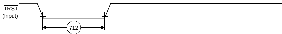
Figure 25. TRST Timing Diagram
