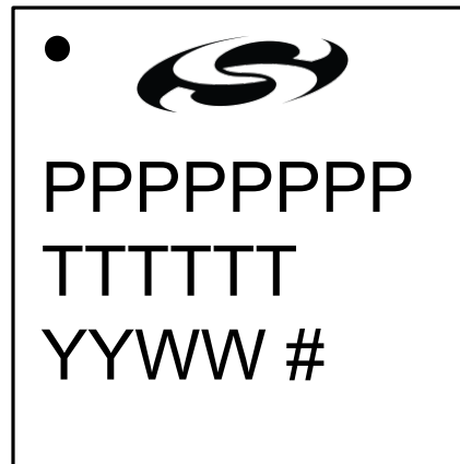
Figure 6.3. QFN28 Package Marking
