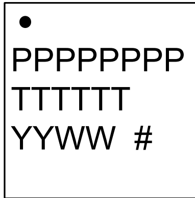
Figure 7.3. QFN24 Package Marking
