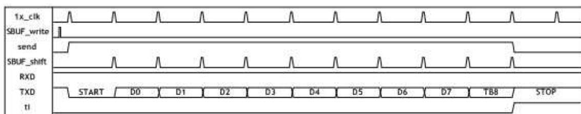
Figure 6.10 Timing Diagram for UART Transmission Mode3
