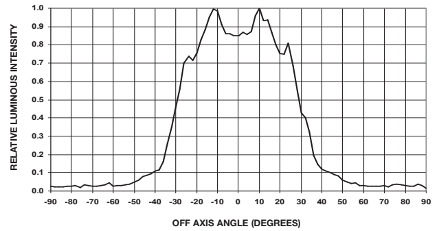
Figure 5e. HPWA(T)-Dx00 Relative Luminous Intensity vs. Off Axis Angle.
