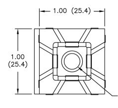
MOUNTING HOLE FOR A #8(M4) FLAT HEAD SCREW
