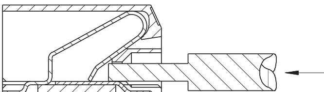
PUSH WIRE INTO HOLE IN FRONT OF CONNECTOR
