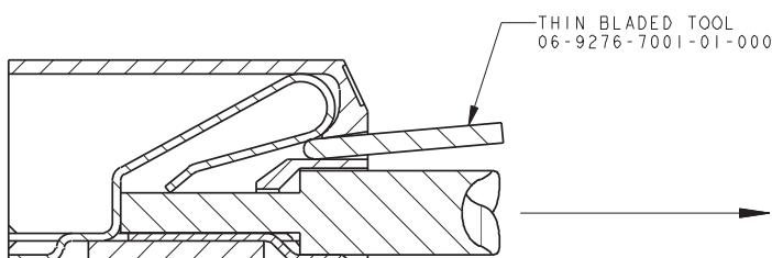
PUSH BLADE (NOT SHARP) INTO SLOT ABOVE WIRE.
