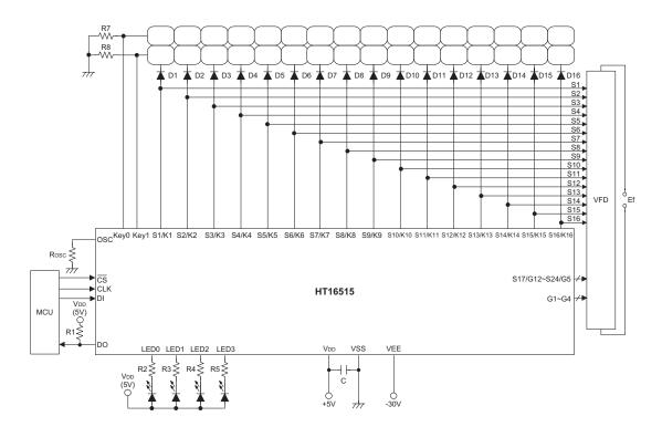
Note:  $R_{OSC}$ =82 $k\Omega$  for oscillator resistor
