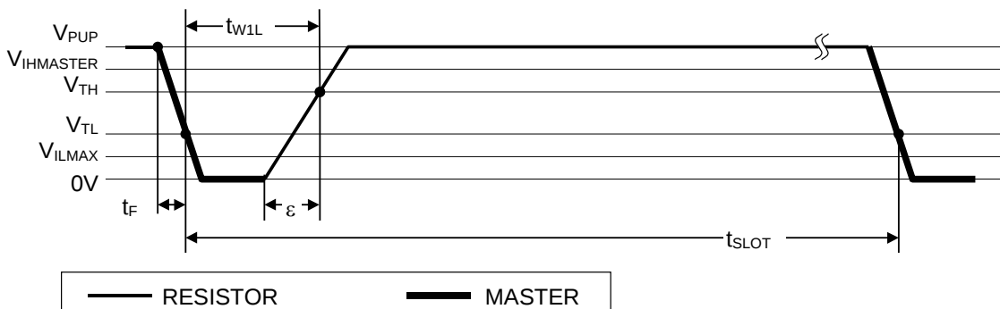
Figure 11. READ/WRITE TIMING DIAGRAM
