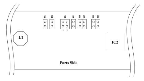
The following table shows the function of No 1 and No 2 of JP4, JP2, JP9. CU40025-UW6J is no reset inputs and M68 CPU bus parallel interface at default setting. Reset input signal is active when it is low.
