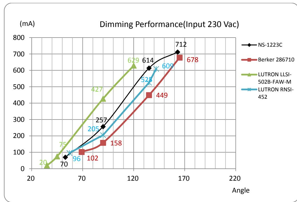
Triac dimming performance is typical as with other models, for specific details on other model performance, please see the Aimtec Triac Dimming Application note at [www.aimtec.com](http://www.aimtec.com)
