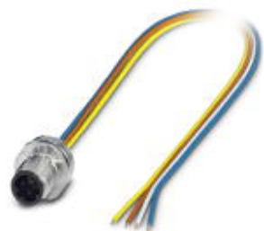
Bus system flat-type plug, PROFINET, 4-position, Plug, straight, M12-SPEEDCON, D-coded, Front mounting, M16 x 1.5, Individual wires, cable length: 0.5 m
