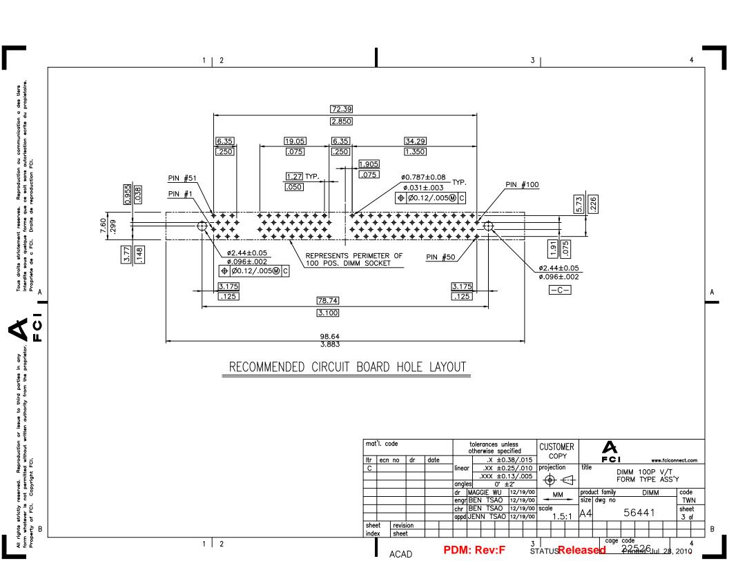
1 | 2 56441 - 🗆 🗆 🗆 🗆 **PLATING** STYLE 1 : FOR UNBUFFERED DRAM, 3.3 VOLT. 2 : FOR UNBUFFERED DRAM, 5.0 VOLT. 3 : FOR DDR DRAM, 2.5 VOLT. CODE CONTACT SOLDERTAIL UNDERPLATE 150µ"(3.81µm) MIN. TIN/LEAD 15μ"(0.38μm) 2 PEG TYPE MIN. GOLD 100μ"(2.54μm) 30μ"(0.76μm) MIN. TIN/LEAD 0 : WITH RETENTION PEG = 3.04/.1203 MIN. GOLD 3μ"(0.076μm) MIN. GOLD 50μ" (1.27μm) MIN. NICKEL OVERALL 150µ"(3.81µm) TAIL LENGTH 6LF MIN. 100% TIN 7LF 15\(\mu^{\mu}(0.38\(\mu\mm)) \\
