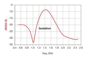
**Note:** Measurements were taken using an Anritsu 4 port VNA; Diplexer was mounted on a custom evaluation board. To reduce systematic errors from the VNA, the coaxial measurement cables, and evaluation board, a Short-Open-Load-Thru (SOLT) calibration was performed, using a custom fabricated calibration substrate. This is the most common coaxial calibration methods.
