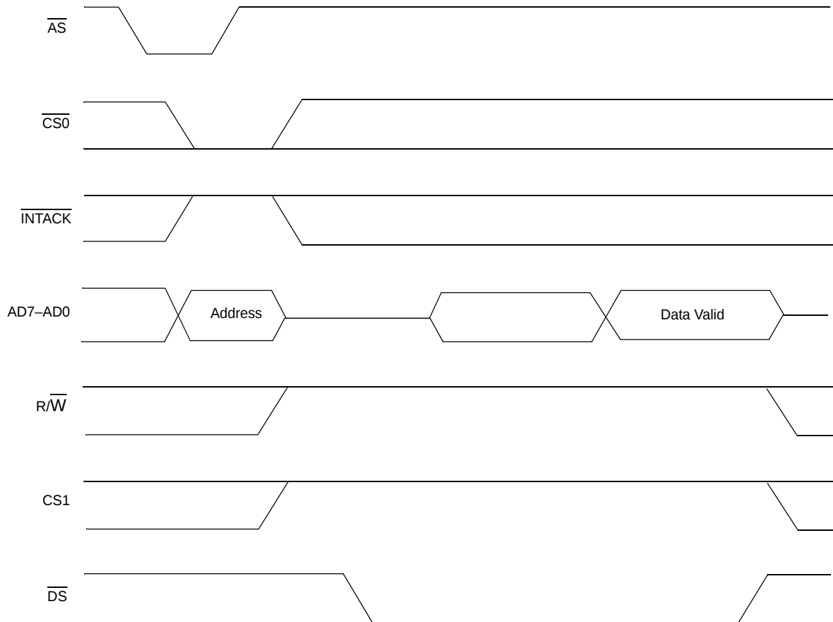
Figure 24. Read Cycle Timing
