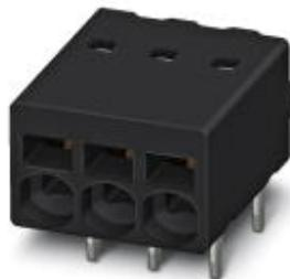
PCB terminal block, nominal current: 6 A, nom. voltage: 160 V, pitch: 2.5 mm, number of positions: 8, connection method: Push-in spring connection, mounting: THR soldering, conductor/PCB connection direction: 0°, color: black
