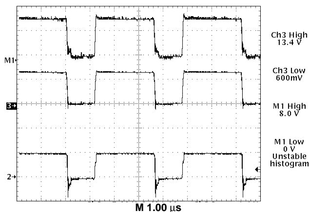
Figure 17. CS5156H Gate Drive Waveforms Depicting Rail to Rail Swing
