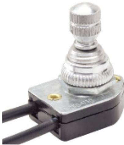
Rotary switch, single pole on-off; 1.5A-125VAC-L, 3A-125VAC, 1A-250VAC; male round bushing 3/8-27 inch long thread; two 6 inch black leads 18AWG AWM TEW 105C 600V, free ends stripped 1/2 inch.
