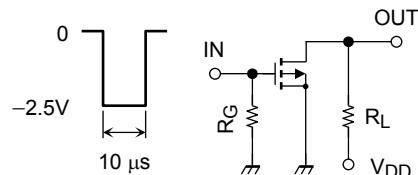
$V_{DD} = -10 V$
