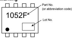
•Note: ● on the lower left of the marking indicates Pin 1
