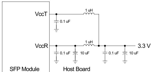
**Example SFP Host Board Schematic**
