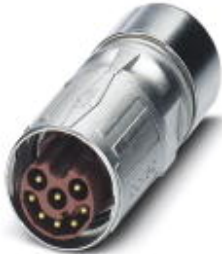
Cable connector, straight, SPEEDCON locking, M17, Number of positions: 17, Type of contact: Male connector, Crimp connection, shielded: Yes, Cable diameter: 5 mm...9 mm
