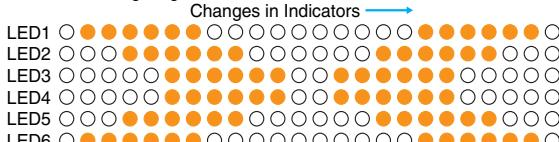
\*2. The flashing speed can be changed in picking display mode (all flashing, elevator-like lighting, or accordion-like lighting) or in external picking display mode. The flashing speed varies with each display mode.
