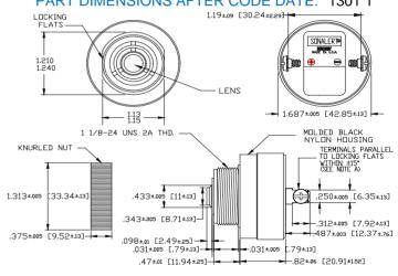
NOTE A: TERMINALS-.032 BRASS TIN PLATED, TAPPED FOR #6-32 SCREW, TWD #6-32 NICKEL PLATED BRASS SCREWS INCLUDED, WILL ACCEPT 1/4' QUICK CONNECT. NOTE B: MOUNTING- REMOVE BLACK PLASTIC NUT AND INSERT THREADED FRONT THROUGH 1.25° HOLE PUNCHED IN PANEL, IF DRIENTATION IS NEEDED, NOTE LOCKING FLATS ON DRAWING, SCREW NUT BACK ON. DO NOT OVERTIGHTEN.
