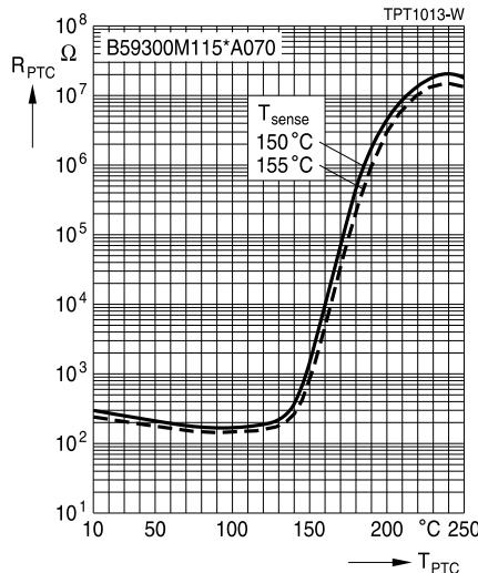
**Sensors****Motor protection, triple sensors****M1300****Characteristics (typical)**
