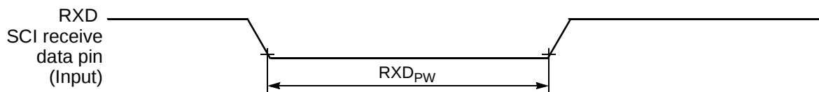
Figure 27. RXD Pulse Width
