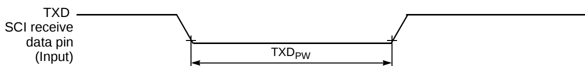
Figure 28. TXD Pulse Width
