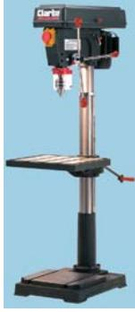
Pedestal drilling machine. Features frontmount no volt release safety switch, emergency stop switch, safety cut out on belt guard, rack and pinion table lift, wet T slot table, depth gauge, work light, chuck and guard. 230V.
