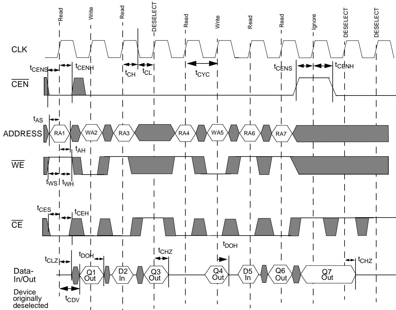
$\overline{WE}$  is the combination of  $\overline{WE}$  &  $\overline{BWS}_x$  to define a Write Cycle (see Write Cycle Description Table).
