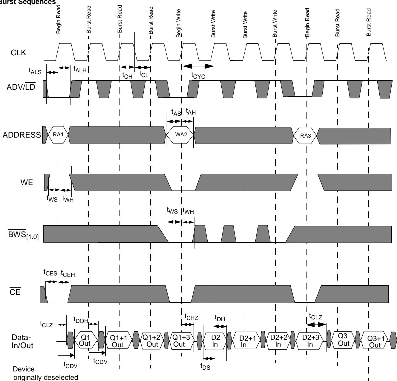
The combination of  $\overline{WE}$  &  $\overline{BWS}_{[1:0]}$  defines a write cycle (see Write Cycle Description Table).
