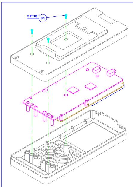
Use the following procedure to remove the meter case.
