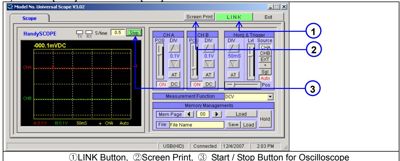
①LINK Button, ②Screen Print, ③ Start / Stop Button for Oscilloscope
