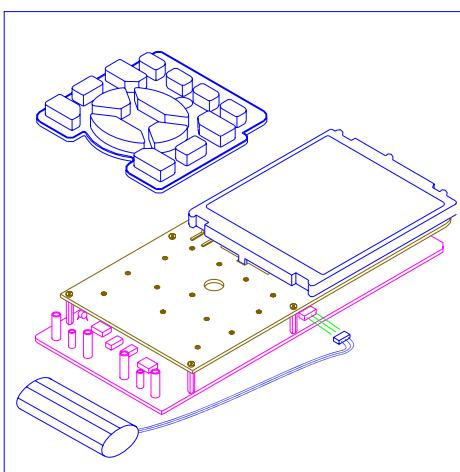
Rotate the PCB Assembly 180 degrees.
