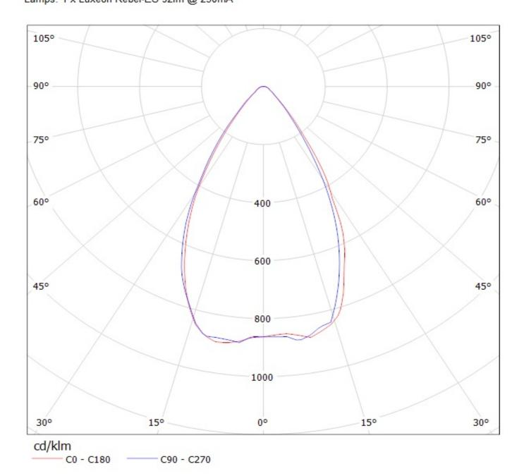
NOTE: The typical divergence will be changed by different color, chip size and chip position tolerance. The typical total divergence is the full angle measured where the luminous intensity is half of the peak value.
