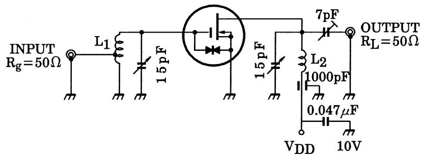
$L_1$ : 1.0 mm $\phi$  silver plated copper wire 4.0 T, 8 mm $\phi$  ID TAP at 1.0 T from coil end
