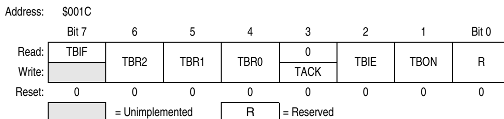
Figure 21-2. Timebase Control Register (TBCR)
