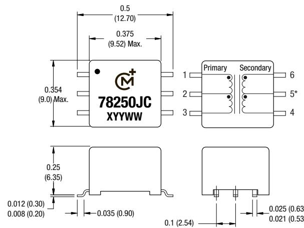
Unless otherwise stated all dimensions in inches (mm)  $\pm 0.01$  (0.25).All pins on a 0.1 (2.54) pitch and within  $\pm 0.01$  (0.25) of true position.
