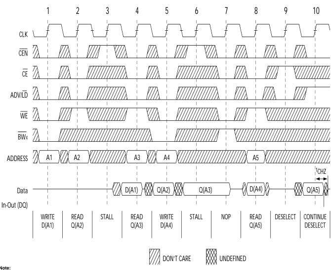
26. The IGNORE CLOCK EDGE or STALL cycle (Clock 3) illustrated CEN being used to create a pause. A write is not performed during this cycle.
