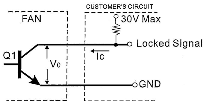
\*Transistor Q1 at "ON" position
