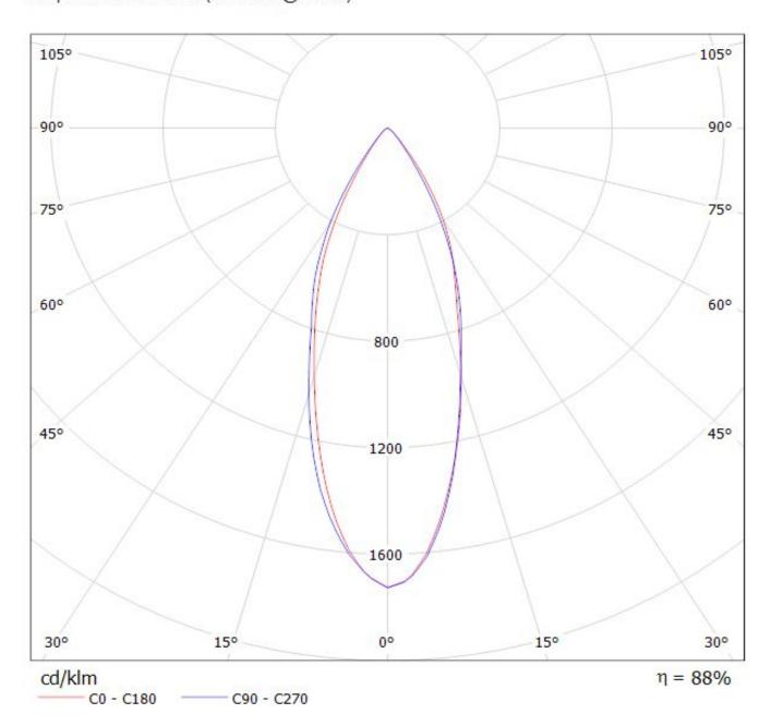
Luminaire: LEDiL Oy FP11124&FP11120\_Lisa2-O\_(SSL80) Eff.80.4% Lamps: 1 x Oslon SSL80 (77.5621lm@250mA)
