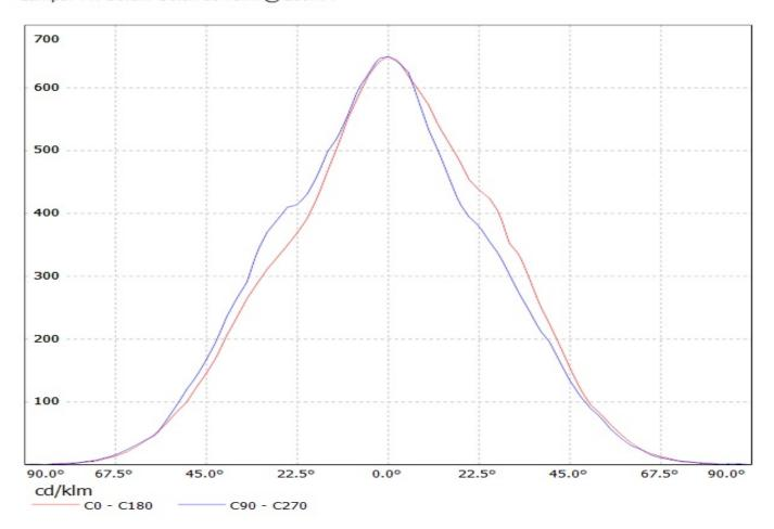
Luminaire: LEDiL Oy FP11002 & FP11082\_LISA2-W\_(SSL80) Eff.87.5% Lamps: 1 x Oslon SSL80 (77.5072lm@250mA)
