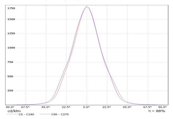
Luminaire: LEDiL Oy FP11124&FP11120\_Lisa2-O\_(SSL80) Eff.80.4% Lamps: 1 x Oslon SSL80 (77.5621lm@250mA)
