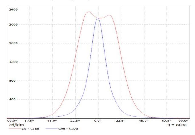
Luminaire: Ledil Oy FP11957 & FP11958\_LISA2-WWW (Osram Oslon 80 79Im @ 250mA) Efficiency=74% Lamps: 1 x Osram Oslon 80 79Im @ 250mA
