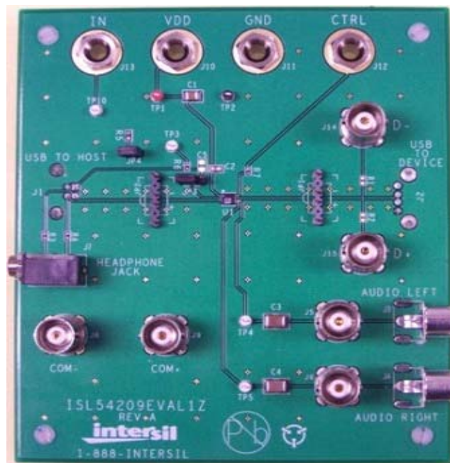
FIGURE 1. ISL54209EVAL1Z EVALUATION BOARD
