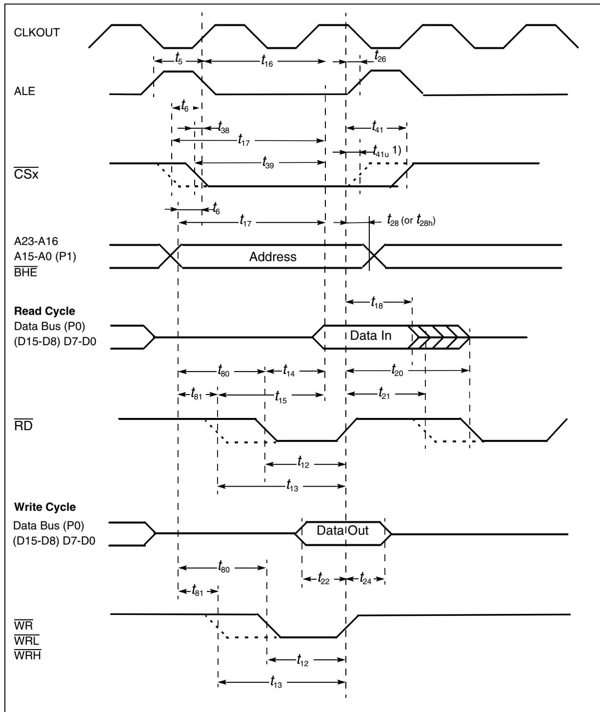
Note: 1. Un-latched CSx =  $t_{41u} = t_{41} - 1$  TCL =  $10.5 + t_F$
