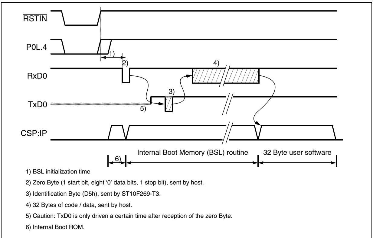
When the ST10F269-T3 has entered BSL mode, the following configuration is automatically set (values that deviate from the normal reset values, are **marked**):
