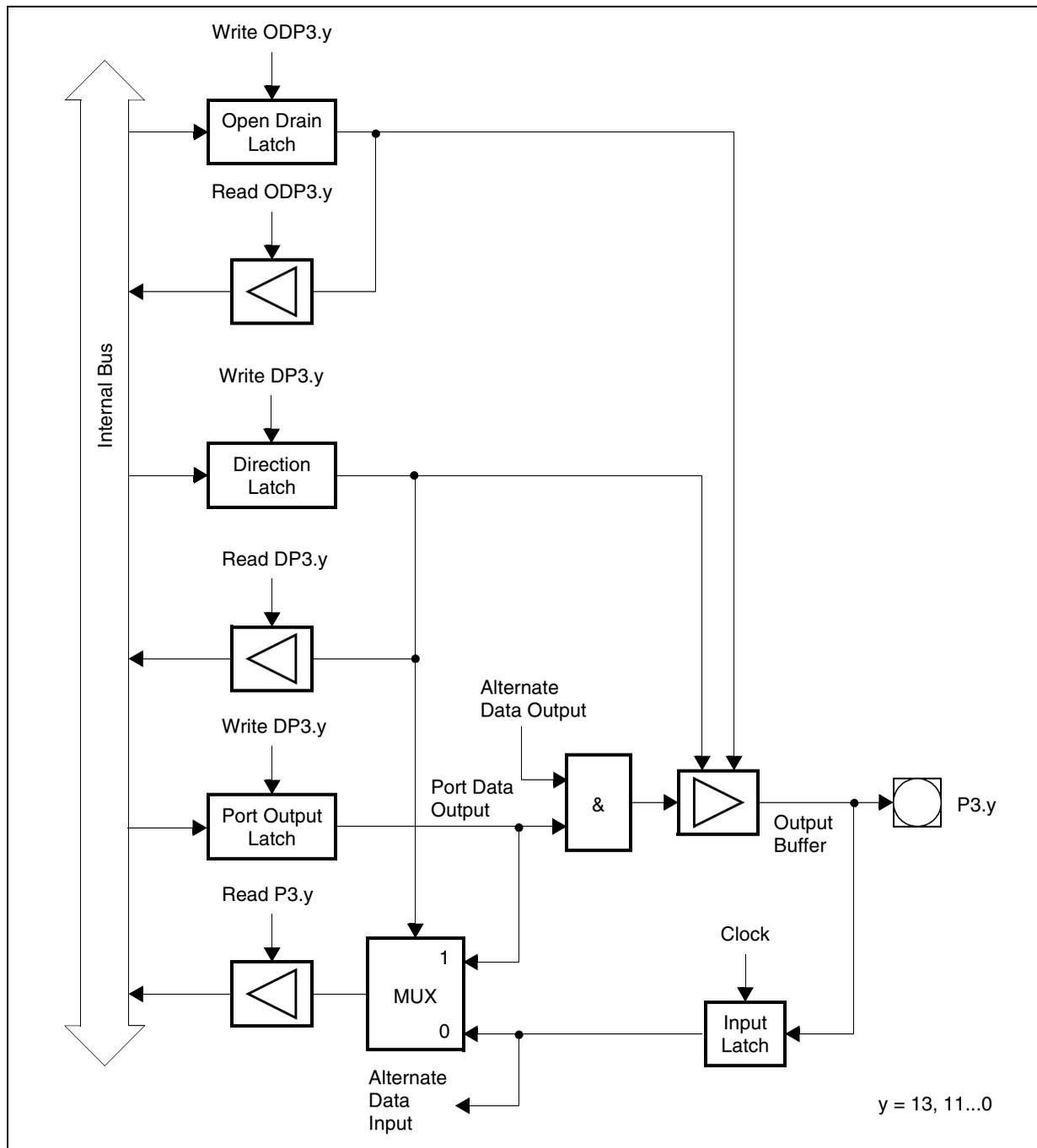
Pin P3.12 ( $\overline{\text{BHE}}/\overline{\text{WRH}}$ ) is another pin with an alternate output function, however, its structure is slightly different.
