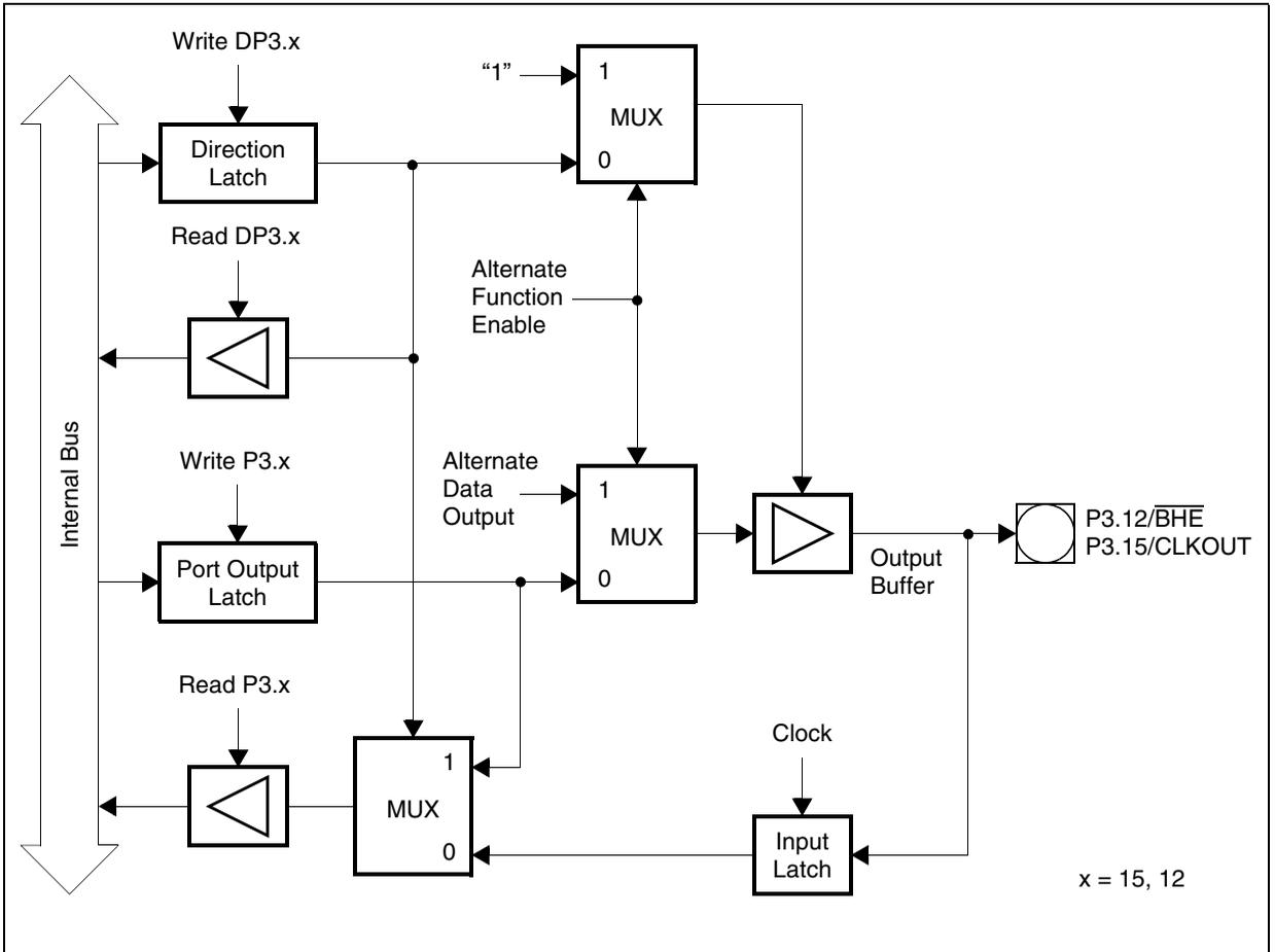
Note: Enabling the  $\overline{\text{BHE}}$  or  $\overline{\text{WRH}}$  function automatically enables the P3.12 output driver. Setting bit DP3.12='1' is not required.
