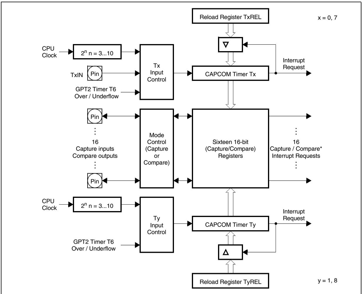
\* The CAPCOM2 unit provides 16 capture inputs, but only 12 compare outputs. CC241 to CC271 are inputs only.
