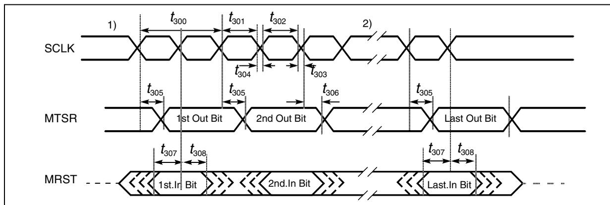
Notes: 1. The phase and polarity of shift and latch edge of SCLK is programmable. This figure uses the leading clock edge as shift edge (drawn in bold), with latch on trailing edge (SSCPH = 0b). Idle clock line is low, leading clock edge is low-to-high transition (SSCPO = 0b).
