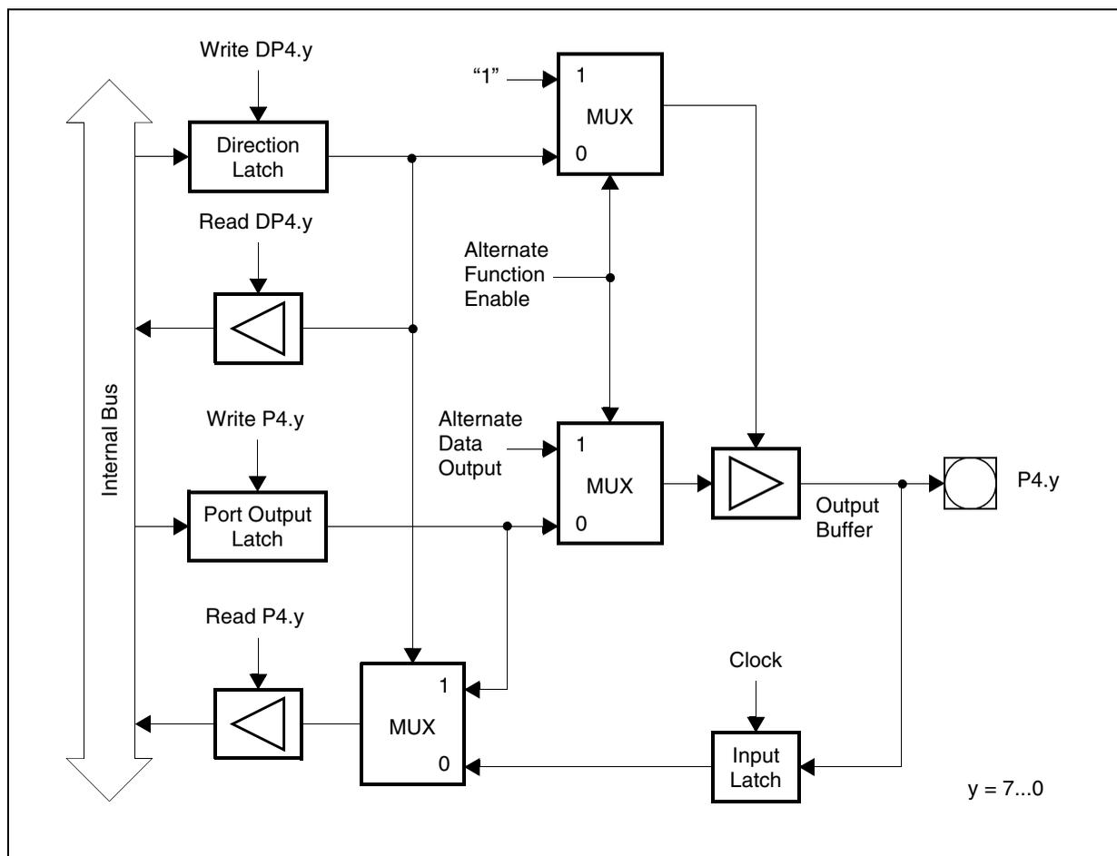
Figure 32 : Block Diagram of P4.4 and P4.5 Pins
