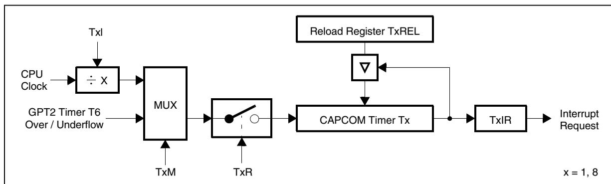
Note: When an external input signal is connected to the input lines of both T0 and T7, these timers count the input signal synchronously. Thus the two timers can be regarded as one timer whose contents can be compared with 32 capture registers.
