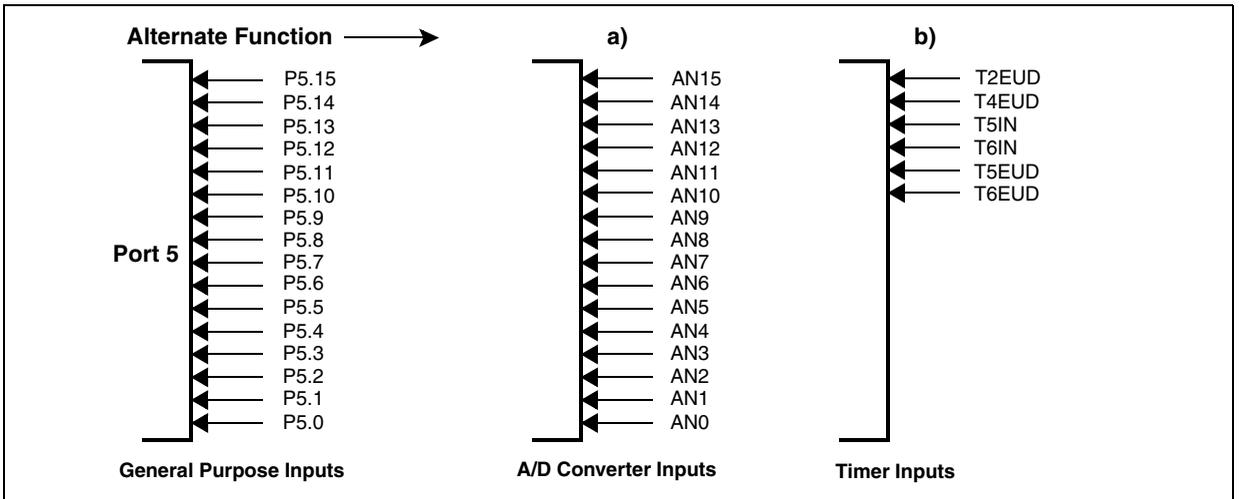
Port 5 pins have a special port structure (see Figure 35), first because it is an input only port, and second because the analog input channels are directly connected to the pins rather than to the input latches.
