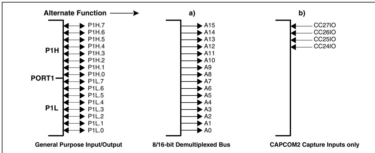
When an external bus mode is enabled, the direction of the port pin and the loading of data into the port output latch are controlled by the bus controller hardware.
