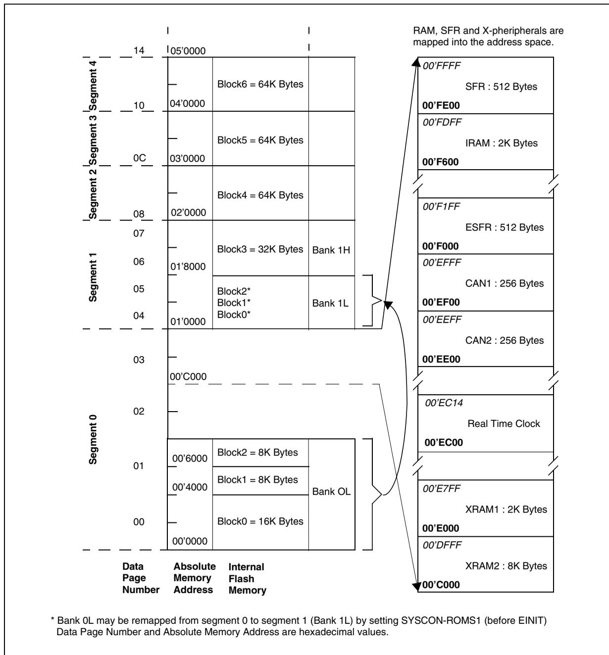
\* Bank 0L may be remapped from segment 0 to segment 1 (Bank 1L) by setting SYSCON-ROMS1 (before EINIT)
