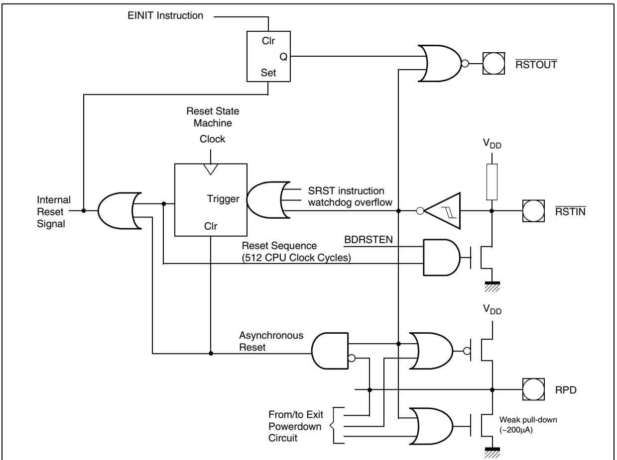
Figure 59 : Minimum External Reset Circuitry
