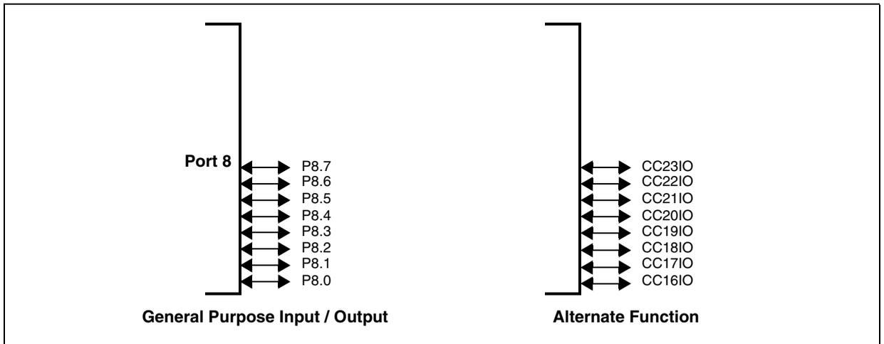
The structure of Port 8 differs in the way the output latches are connected to the internal bus and to the pin driver (see Figure 43). Pins P8.7...P8.0
