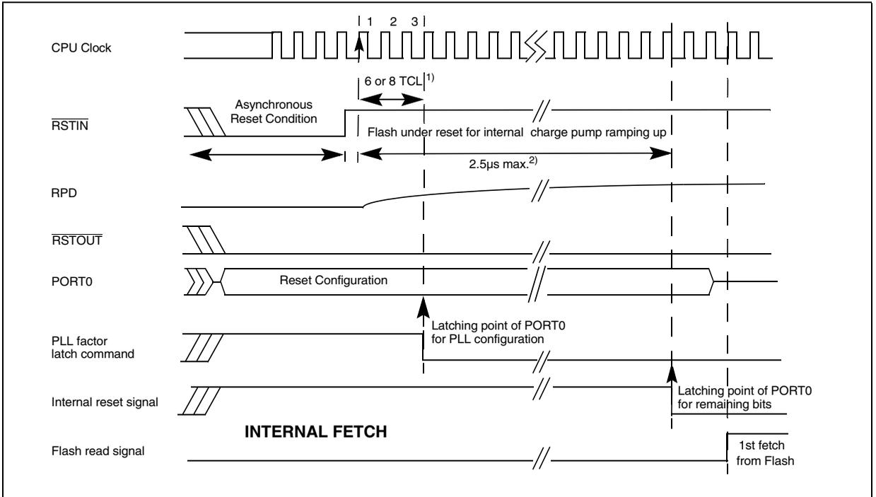
Note: 1)  $\overline{RSTIN}$  rising edge to internal latch of PORT0 is 3 CPU clock cycles (6 TCL) if the PLL is bypassed and the prescaler is on ( $f_{CPU} = f_{XTAL} / 2$ ), else it is 4 CPU clock cycles (8 TCL).
