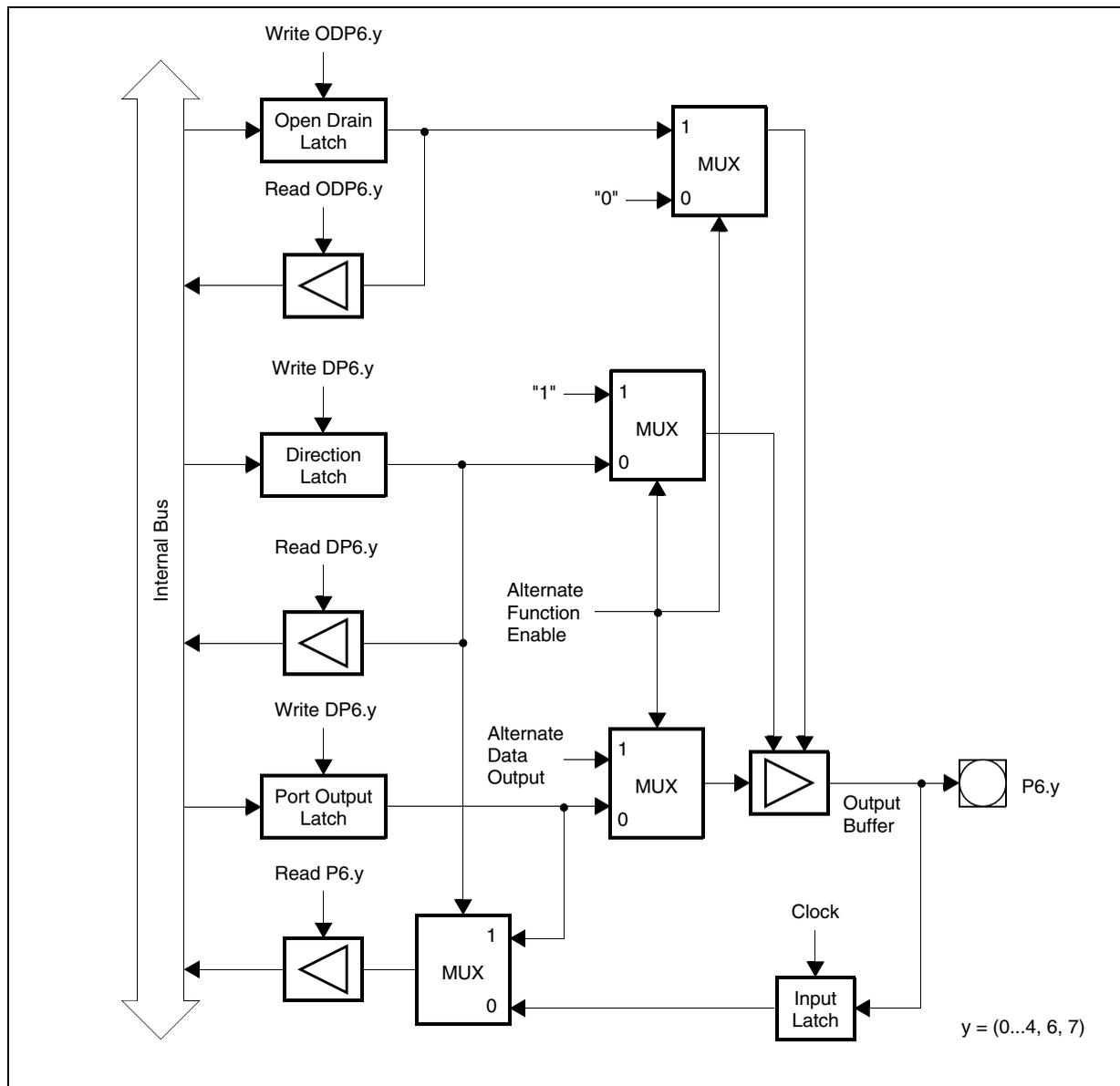
Figure 38 : Block Diagram of Pin P6.5 ( $\overline{\text{HOLD}}$ )
