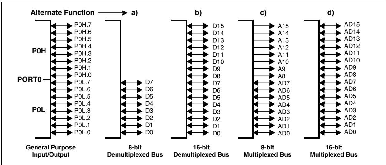
When an external bus mode is enabled, the direction of the port pin and the loading of data into the port output latch are controlled by the bus controller hardware.
