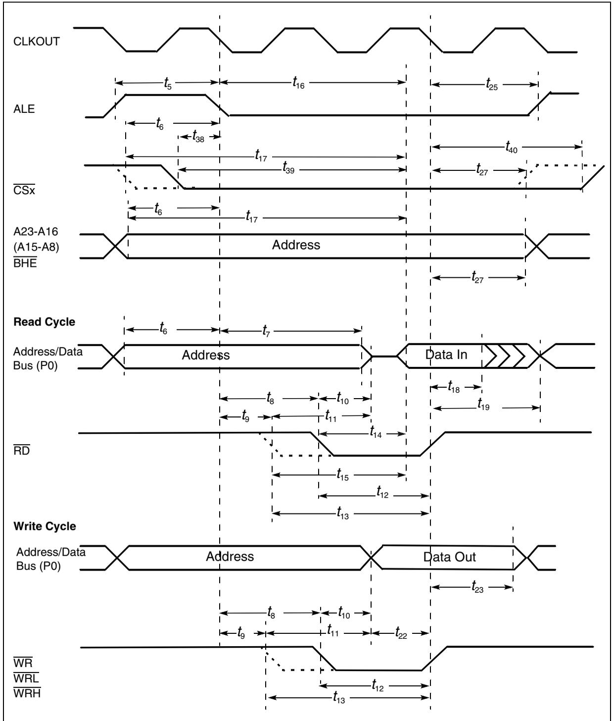
**Figure 72** : External Memory Cycle: Multiplexed Bus, With / Without Read / Write Delay, Normal ALE, Read / Write Chip Select
