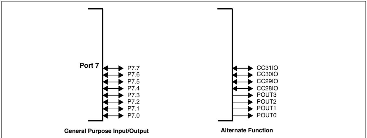
The structure of Port 7 differs in the way the output latches are connected to the internal bus and to the pin driver. Pins P7.3...P7.0 (POUT3...POUT0)
