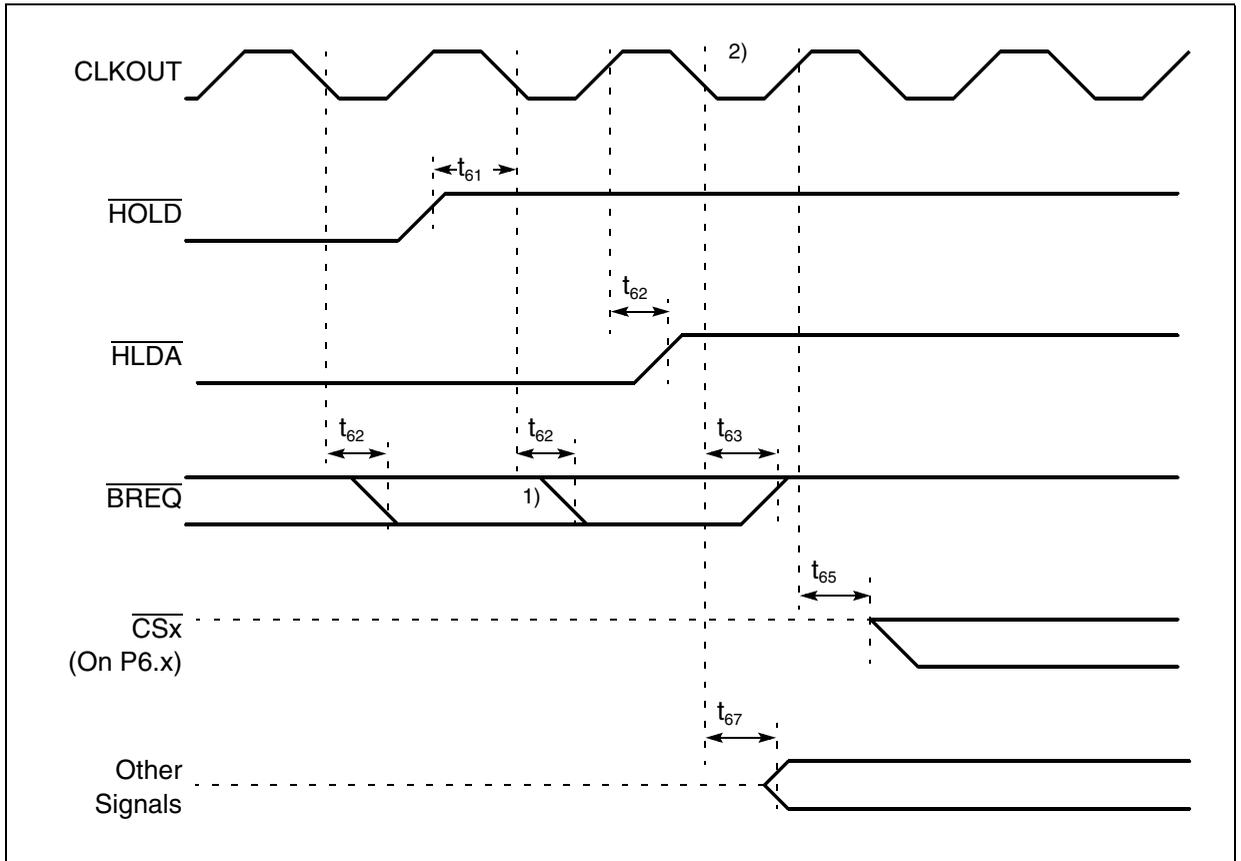
Notes: 1. This is the last chance for  $\overline{BREQ}$  to trigger the indicated regain-sequence. Even if  $\overline{BREQ}$  is activated earlier, the regain-sequence is initiated by  $\overline{HOLD}$  going high. Please note that  $\overline{HOLD}$  may also be de-activated without the ST10F269-T3 requesting the bus.
