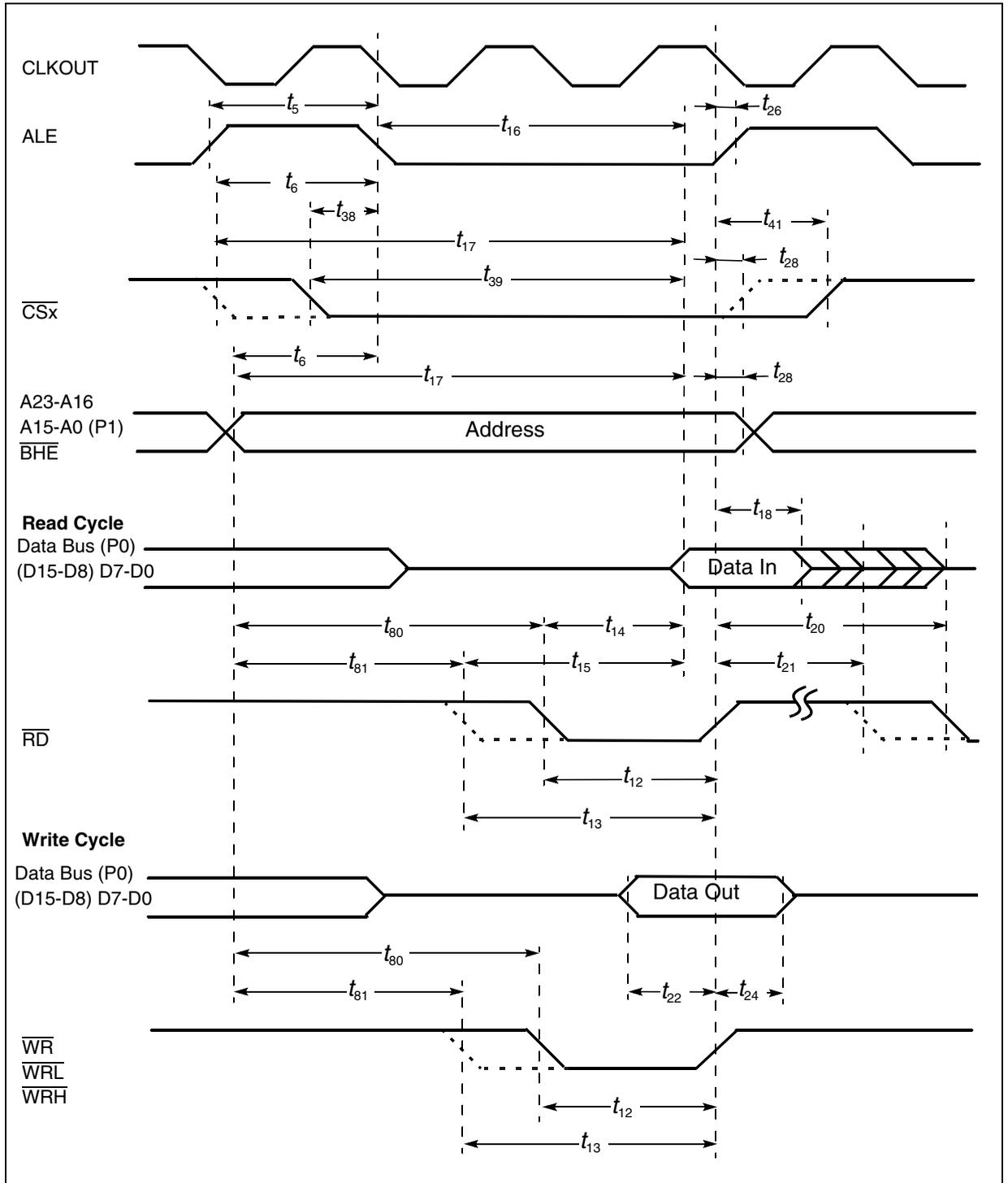
**Figure 76** : External Memory Cycle: Demultiplexed Bus, With / Without Read / Write Delay, Normal ALE, Read / Write Chip Select
