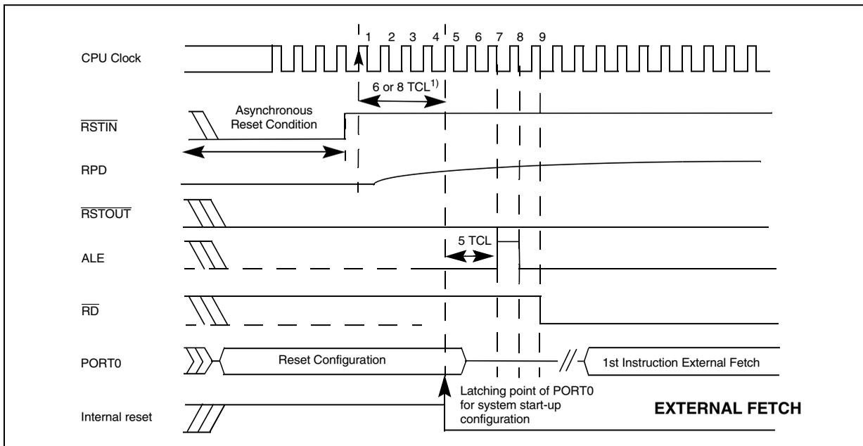
Note: 1)  $\overline{RSTIN}$  rising edge to internal latch of PORT0 is 3 CPU clock cycles (6 TCL) if the PLL is bypassed and the prescaler is on ( $f_{CPU} = f_{XTAL} / 2$ ), else it is 4 CPU clock cycles (8 TCL).
