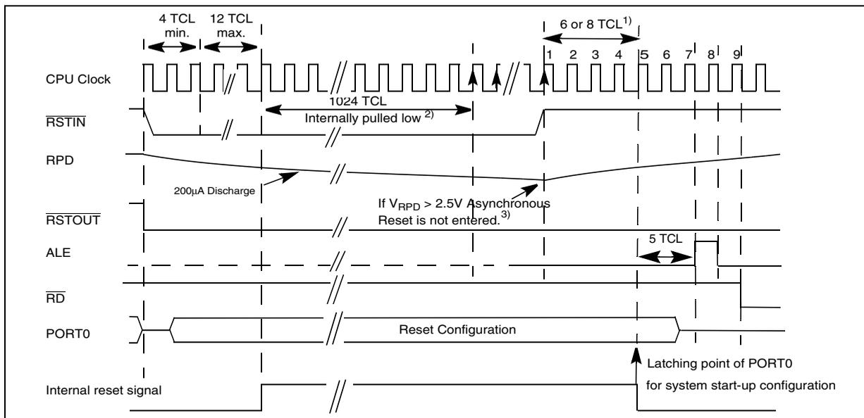
Note 1)  $\overline{\text{RSTIN}}$  rising edge to internal latch of PORT0 is 3 CPU clock cycles (6 TCL) if the PLL is bypassed and the prescaler is on ( $f_{\text{CPU}} = f_{\text{XTAL}} / 2$ ), else it is 4 CPU clock cycles (8 TCL).
