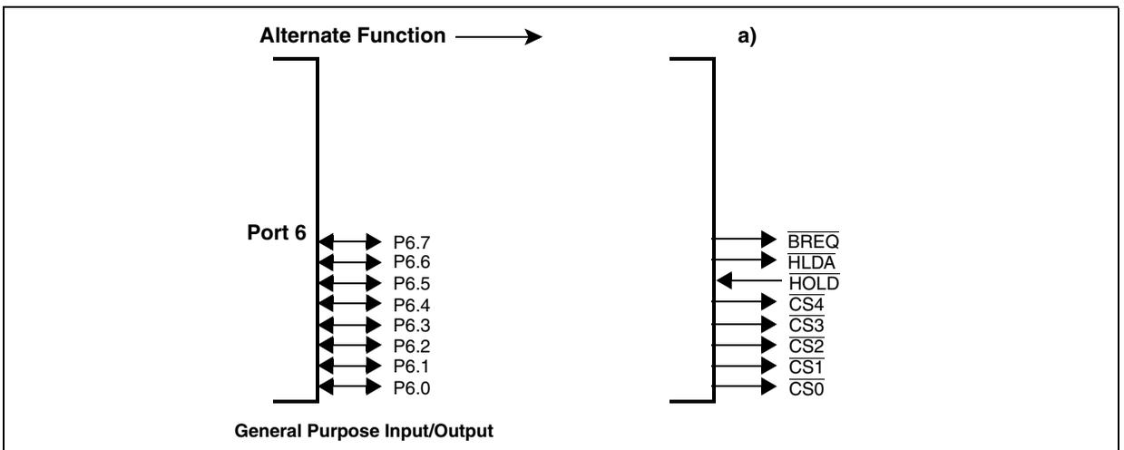
The chip select lines of Port 6 have an internal weak pull-up device. This device is switched on during reset. This feature is implemented to drive the chip select lines high during reset in order to avoid multiple chip selection.
