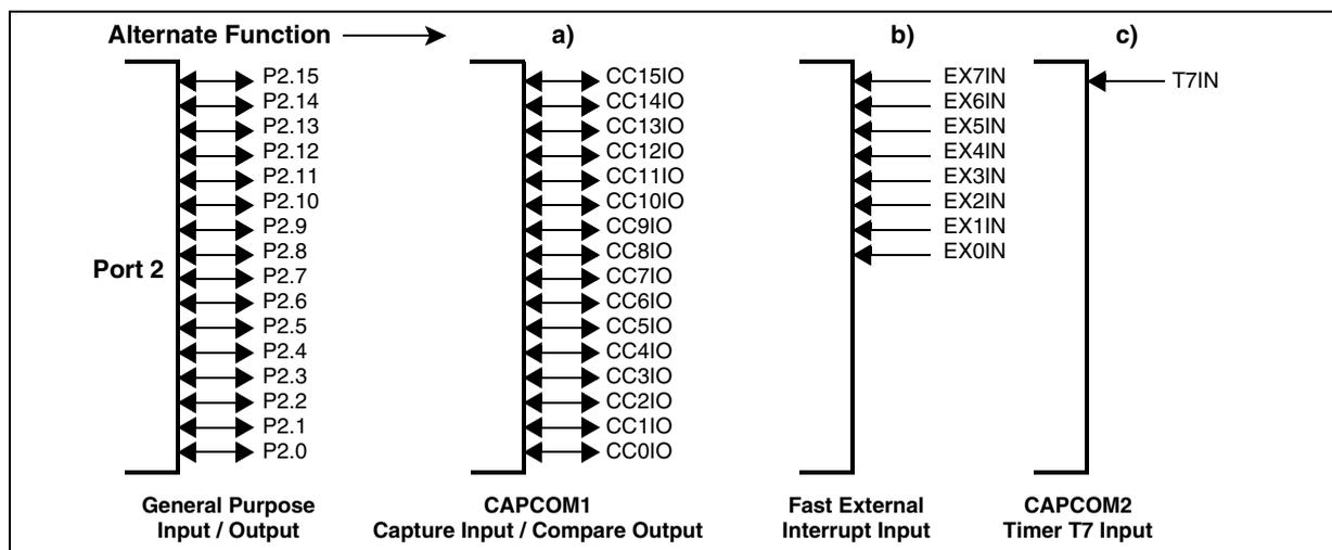
The pins of Port 2 combine internal bus data with alternate data output before the port latch input.
