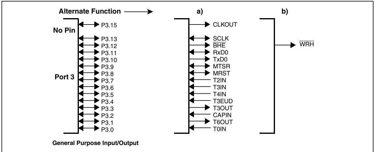
The structure of the Port 3 pins depends on their alternate function (see figures 28 and 29). When the on-chip peripheral associated with a Port 3 pin is configured to use the alternate input function, it reads the input latch, which represents the state of the pin, via the line labeled “Alternate Data Input”. Port 3 pins with alternate input functions are: T0IN, T2IN, T3IN, T4IN, T3EUD and CAPIN.
