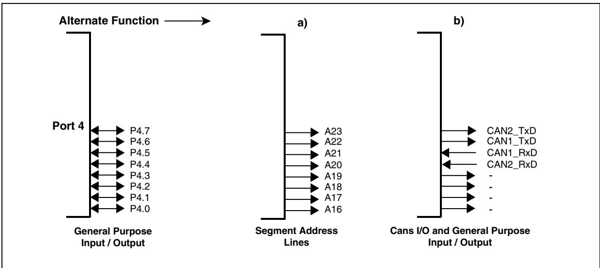
Figure 31 : Block Diagram of a Port 4 Pin
