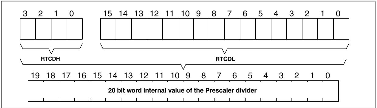
Bit 15 to bit 4 of RTCPH and RTCDH are not used. When reading, the return value of those bit will be zeros.
