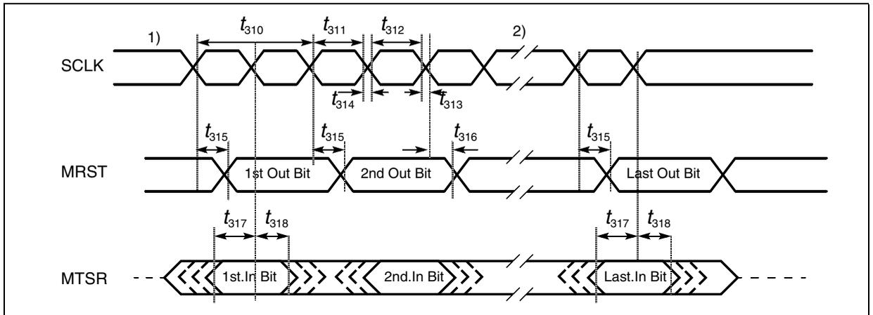
Notes: 1. The phase and polarity of shift and latch edge of SCLK is programmable. This figure uses the leading clock edge as shift edge (drawn in bold), with latch on trailing edge (SSCPH = 0b). Idle clock line is low, leading clock edge is low-to-high transition (SSCPO = 0b).
