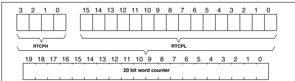
The value stored into RTCPH, RTCPL is called RTCP (coded on 20-bit). The dividing ratio of the Prescaler divider is: ratio = 64 x (RTCP)
