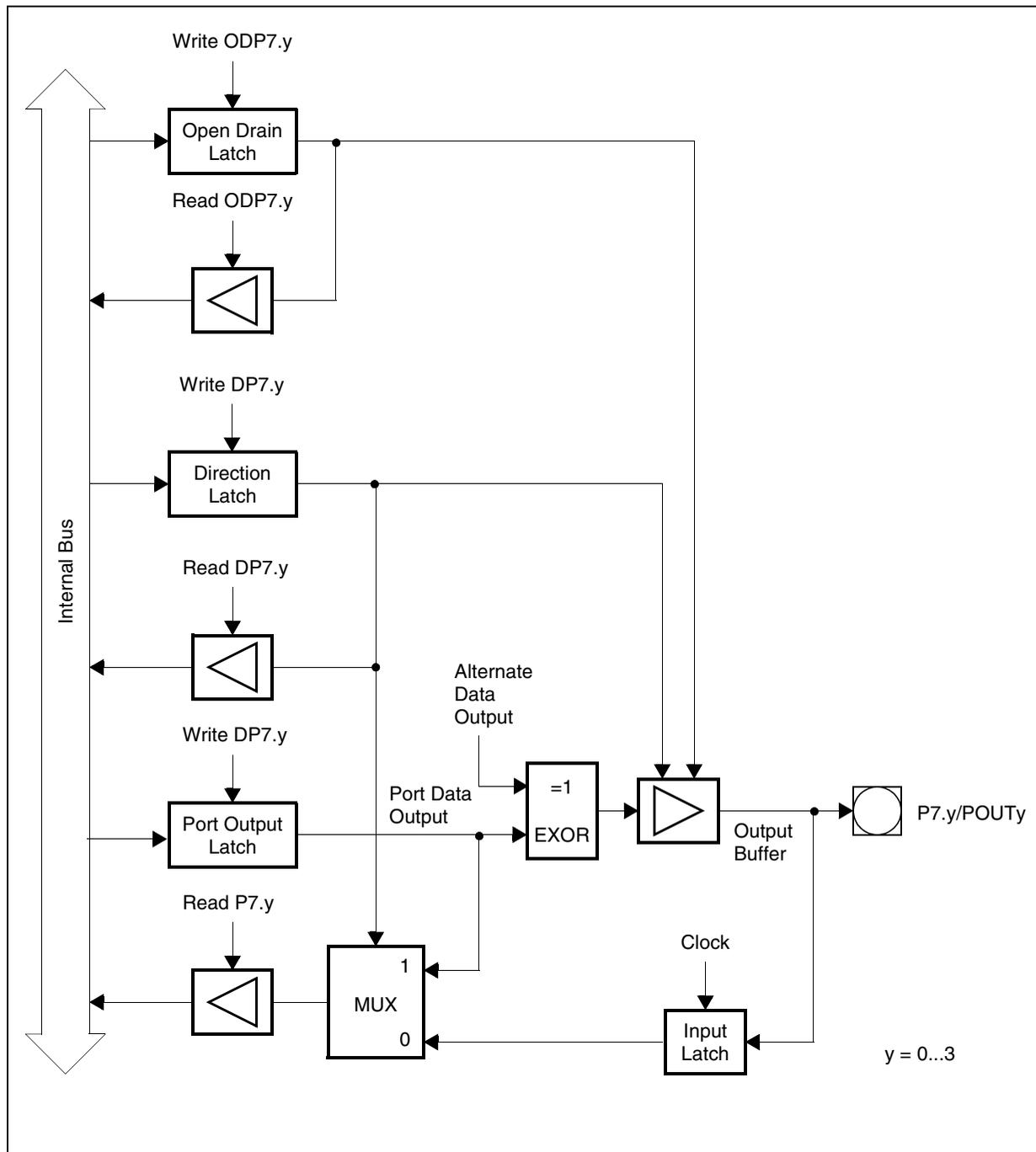
Figure 41 : Block Diagram of Port 7 Pins P7.7...P7.4
